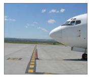
An Aircraft Parking Boundary Line is a single yellow broken line, often parallel to the Apron Taxiway and is used to outline aircraft parking pads. Aircraft are parked behind Aircraft Parking Boundary Lines to ensure they are safely separated and clear of taxiing aircraft.
