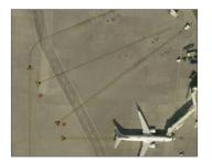
A long single solid yellow line in the middle of an aircraft operational stand that guides aircraft into the parking position. The nose wheel of the aircraft is centered on these lines to ensure the wings do not hit any known obstructions. On the end nearest to the passenger loading bridge there are markings to indicate where the nose wheel of specific aircraft should STOP for the aircraft door to meet the bridge properly. On the opposite end is the number of the operational stand/gate.
