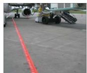
A single red line outlines the boundary of the bridge movement area. Parking is not allowed within the marked area where the bridge can travel unless the aircraft is parked on gate and the vehicle is being used to actively service that aircraft.
