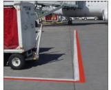
Vehicle & GSE Staging and Parking Area Boundary Lines are parallel solid white and red lines that define the areas intended for use to stage or park ground service equipment and are intended to provide safe separation from aircraft at an operational stand. These lines take into account the wingspan of aircraft. Approved vehicle parking is on the white side of the line.
