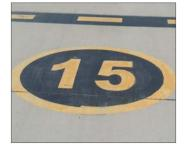
Geographical Position Fix Markings (also called 'Spots') are yellow circles with a number inside and a broken yellow line nearby. These 'Spots' are on the Apron near the exits to Taxiways and are used by Air Traffic Control (ATC) to help direct aircraft taxiing and aircraft under tow transition between the Apron and a Taxiway. The broken yellow line at a 'Spot' acts as a preliminary Hold Line for aircraft exiting the Apron.
