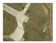
The protected area of a surface designated for the landing and take-off of aircraft. This protected area runs between the extended runway Hold Lines on each side and inside the localizer antenna arrays on each end of the runway. ATC must ensure this area is clear before clearing an aircraft to land or take-off on that runway.
