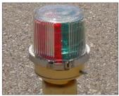
Runway Threshold Lights are two-sided lights, half red, half-green, and are used at the threshold of a Runway. The red half faces the Runway to indicate the end of the Runway and the green half faces the approach for the pilot to see when coming in to land an aircraft.
