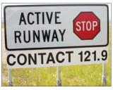
These signs are designed to control traffic entering the threshold of Runway 26. DA, DAS and DAW AVOP holders are not allowed past this sign.
