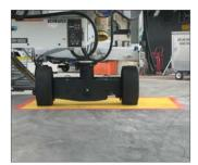
A yellow rectangle outlined in red indicates the area on the Apron where a bridge's wheels are parked when the bridge is not in use. Parking is not allowed in this area.
